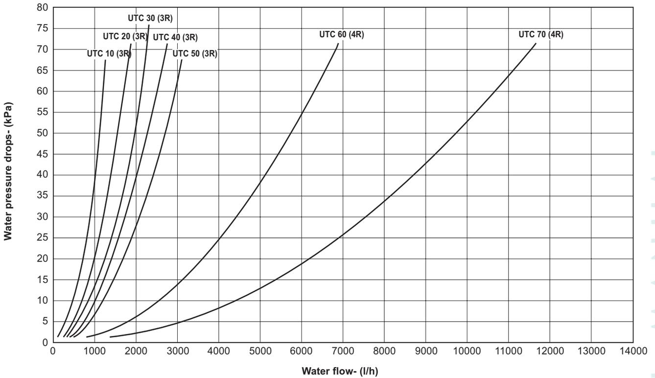
**AUXILIARY COIL** (Ref. Water medium temperature= 65° C)
