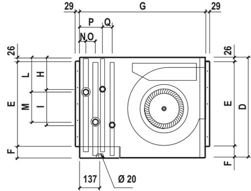
**GENERAL DIMENSIONS OF DUCTABLE AIR TREATMENT UNITS - 4 PIPE SYSTEM**
