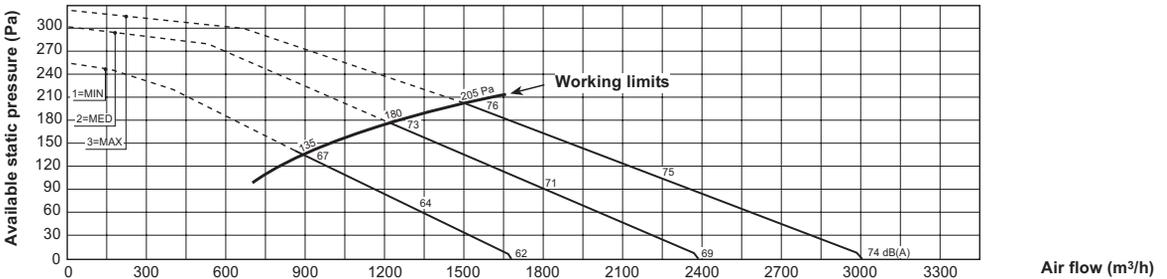
The value indicated with min, med, .max, concern the 3 standard speeds set at the factory.
