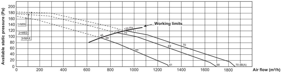
The value indicated with min, med, .max, concern the 3 standard speeds set at the factory.
