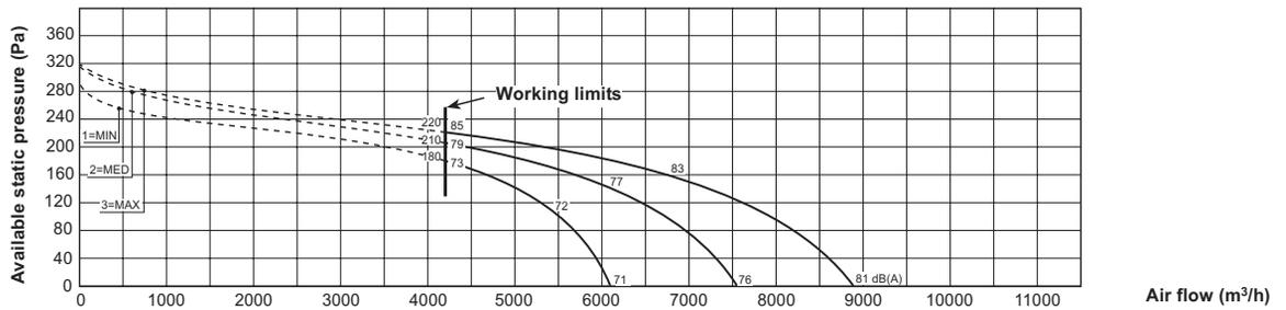
The value indicated with min, med, .max, concern the 3 standard speeds set at the factory.
